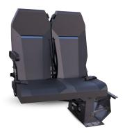
Mid-Back 3-Point Foldaway Add space versatility. Gas shock assisted lift and easy to use foot pedal. Mid-back styling and height compliments our hi-back.
